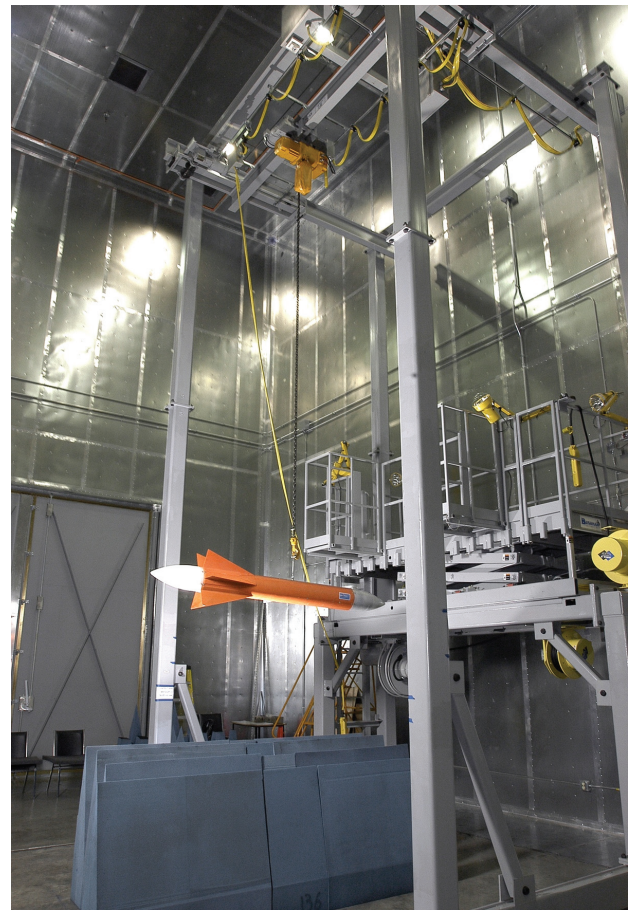
FIGURE 2. Gantry/crane system used in moving large test objects and support crew into the compact range chamber. The suspended object is a towed target frequently used for aircraft interceptor tests.
